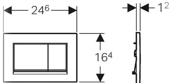
Dimensions: All measurements are in millimetres and are subject to normal manufacturing variations.
