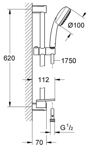
Dimensions: All measurements are in millimetres and are subject to normal manufacturing variations.
