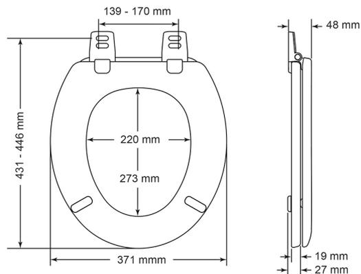
Dimensions: All measurements are in millimetres and are subject to normal manufacturing variations.
