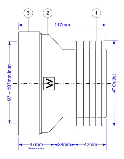
\*WC-INLET Seal has been tested to EN681
