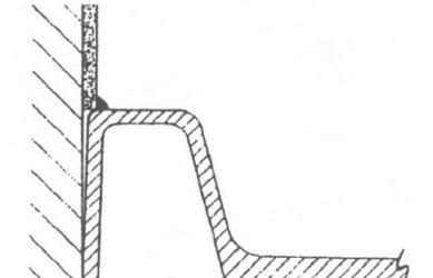
**Important:** This product must be bedded on a weak 5:1 sand/cement mix on a solid base of either concrete or marine ply in all installations. This smoothes out any undulations between the floor and the tray base.
